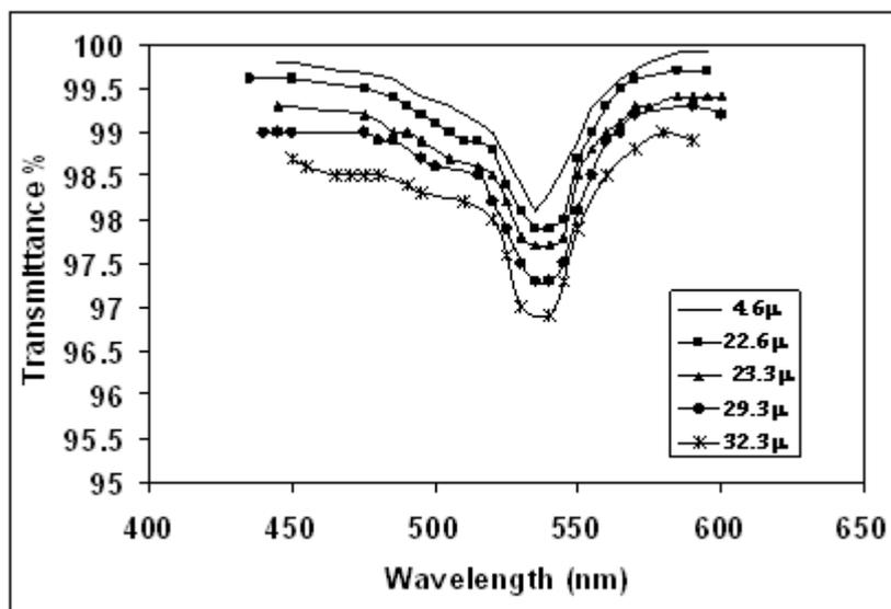
**Figure (1):** Transmittance spectrum for membranes of Rhodamine 6G mixed with epoxy resin at concentration ( $3 \times 10^{-5}$  mol/l) and different thickness.
