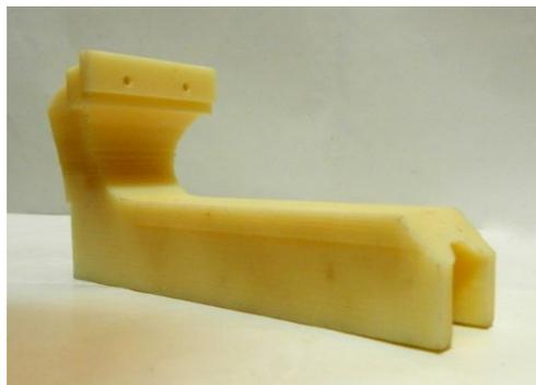
**Fig.5.4** Movable jaw manufactured on RPT machine
