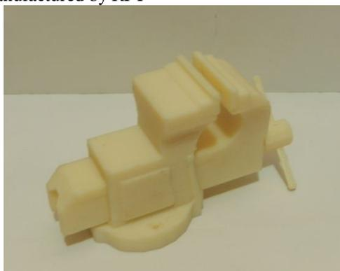
**Fig.5.7** Assembly of movable jaw and modified fixed jaw
