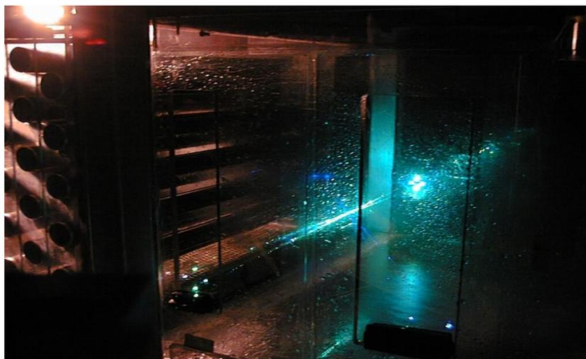
**Figure 4** The PDA measurement volume produced by the intersection of 3 pairs of laser beams
