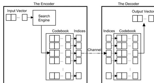
**Figure 1:** The Encoder and decoder in a vector quantize technique. Given an input vector, the closest codeword is found and the index of the codeword is sent through the channel. The decoder receives the index of the codeword, and outputs the codeword.
