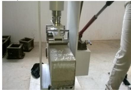
**Figure.6.3** Flexural Strength Test
