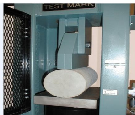
Figure.6.2 Split Tensile Test
