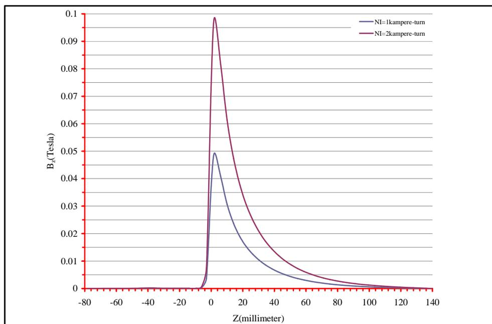
**Figure 5** The axial flux density distribution as a function of axial distance Z of proposed asymmetric lens at NI 1k(ampere-turn) , and 2k(ampere-turn)
