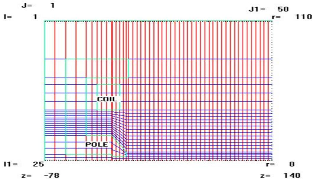
**Figure 3** The produced mesh grid of proposed asymmetric lens
