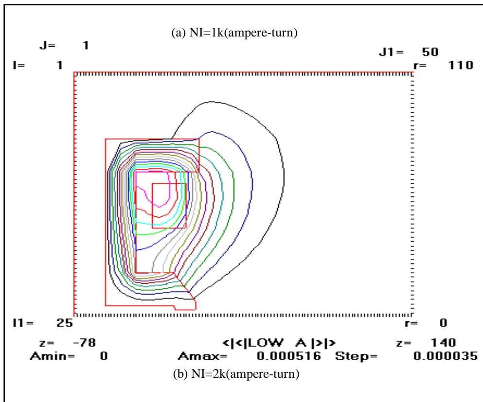
**Figure 4** The magnetic flux lines throughout the iron circuit and coil windings of proposed asymmetric lenses at excitations (a) 1k(ampere-turn), and (b) 2k(ampere-turn)
