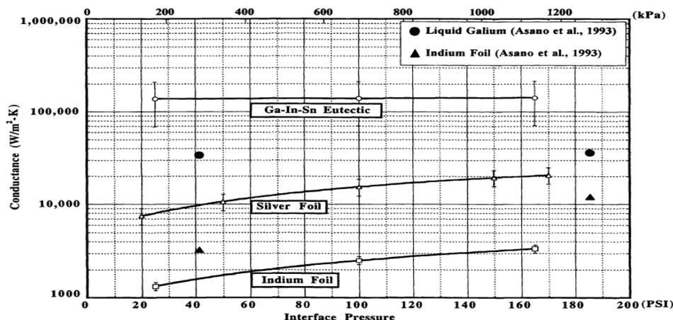
**Figure 2.1** Variation of thermal contact conductance with pressure across a silicon-copper interface with indium foil, silver foil, or an In-Ga-Sn eutectic <sup>[8]</sup>
