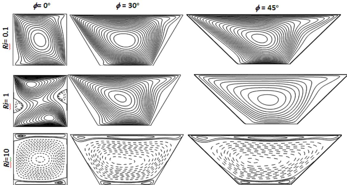
Figure 2 Streamlines for various Richardson numbers and cavity angles at Ha=0
