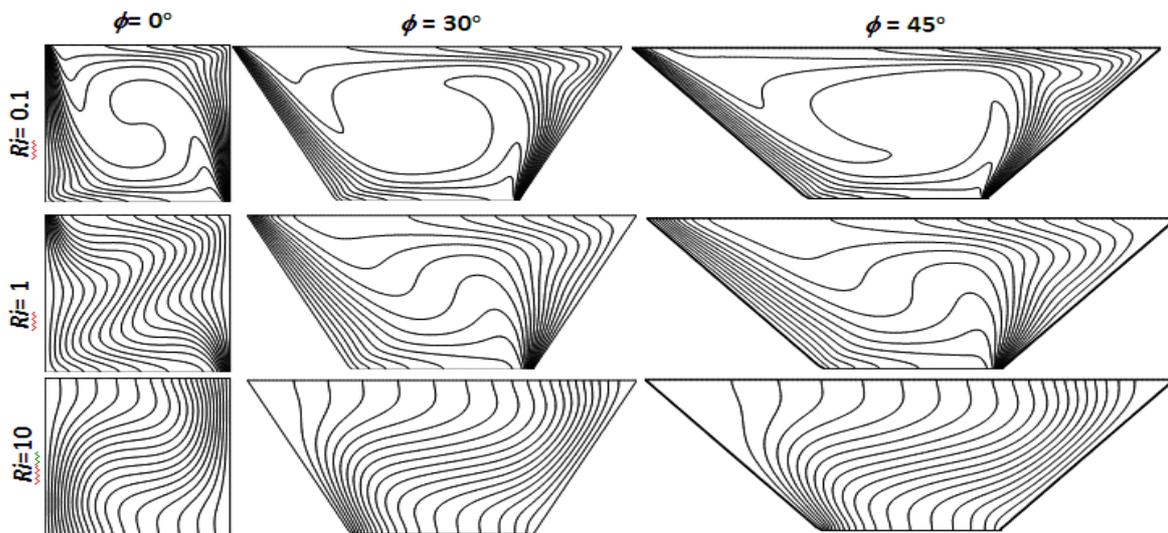
Figure 3 Isotherms for various Richardson numbers and cavity angles at Ha=0
