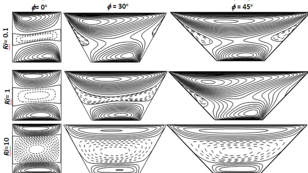
Figure 4 Streamlines for various Richardson numbers and cavity angles at Ha=25
