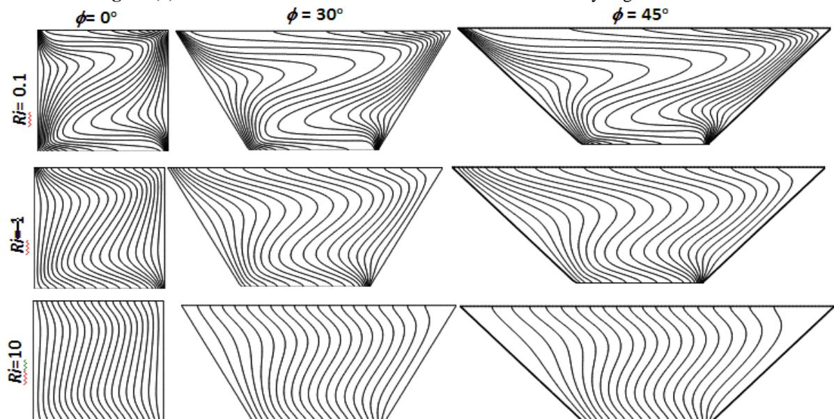
Figure (7) Isotherms for various Richardson numbers and cavity angles at Ha=50
