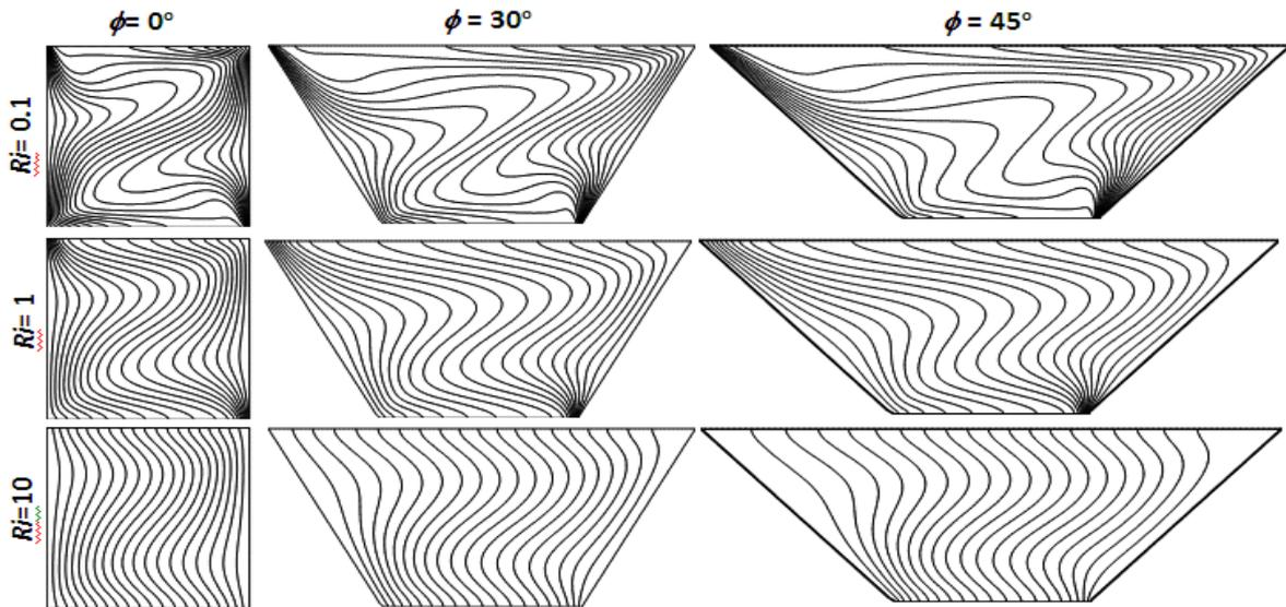
Figure 5 Isotherms for various Richardson numbers and cavity angles at Ha=25
