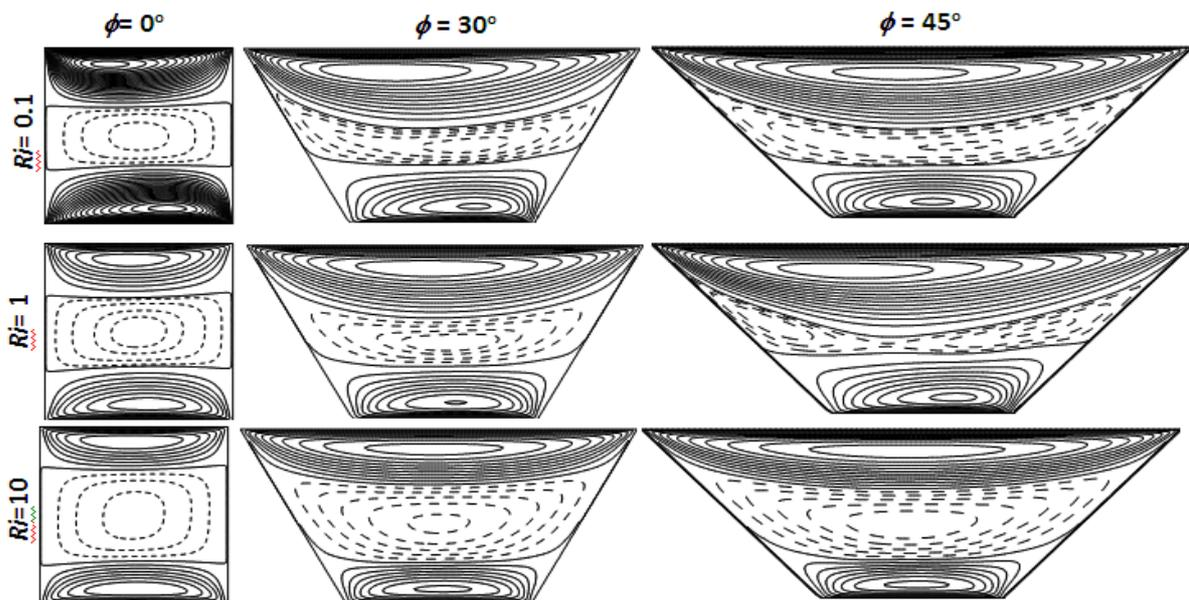
Figure (6) Streamlines for various Richardson numbers and cavity angles at Ha=50
