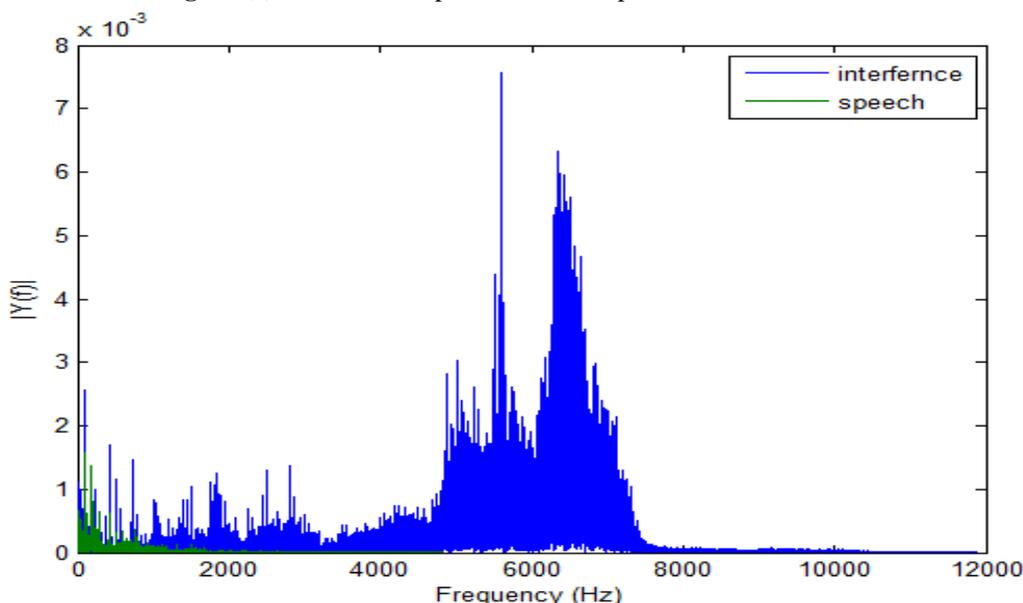
**Figure (2)** Frequency spectrum of both the speech and interference.
