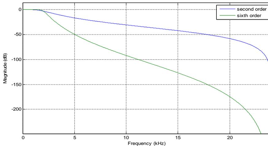
**Figure (3)** Magnitude frequency response of Butterworth low-pass filter for filter order 2<sup>nd</sup> and 6<sup>th</sup>
