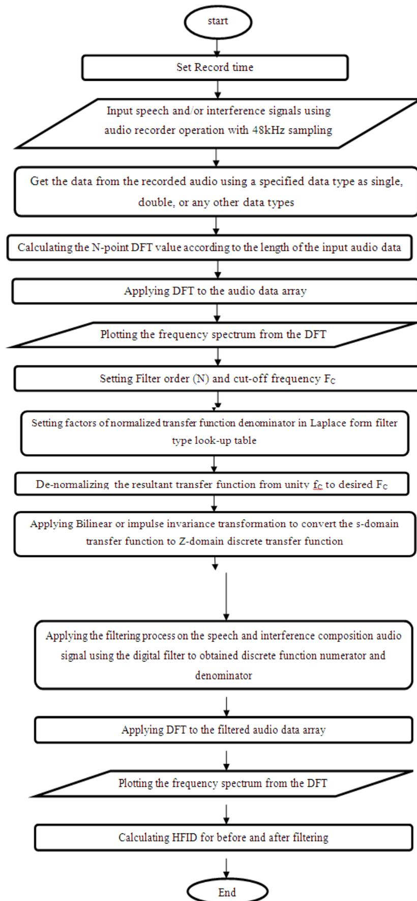
a) **Figure (5)** Flowchart describing digital filter coefficients construction using Bilinear & impulse invariance methods.
