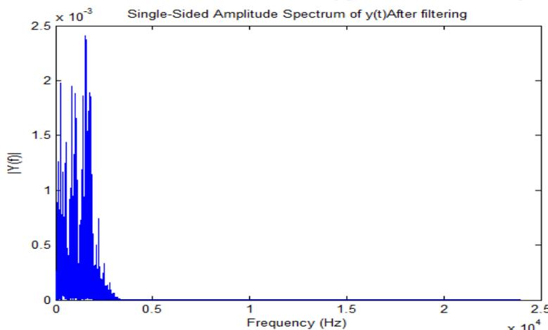
**Figure (6)** Frequency spectrum represents the filtering results of the speech and interference spectrum shown in Figure (4.3) using 6<sup>th</sup> order Butterworth digital filter.
