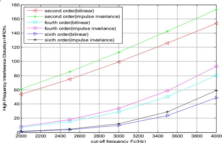
**Figure (7)** Effect of changing filter cut-off frequency on the HFID% of Butterworth digital filter under two design methods
