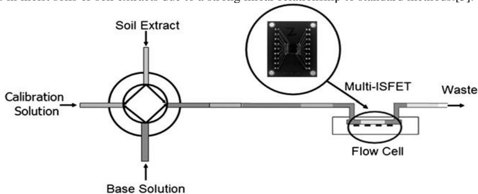
**Fig.2** Shows a schematic of an ion-selective field effect transistor (ISFET)
