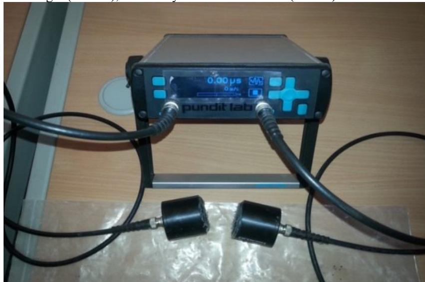
Fig (3.5) shows the ultra-sonic pulse apparatus.
