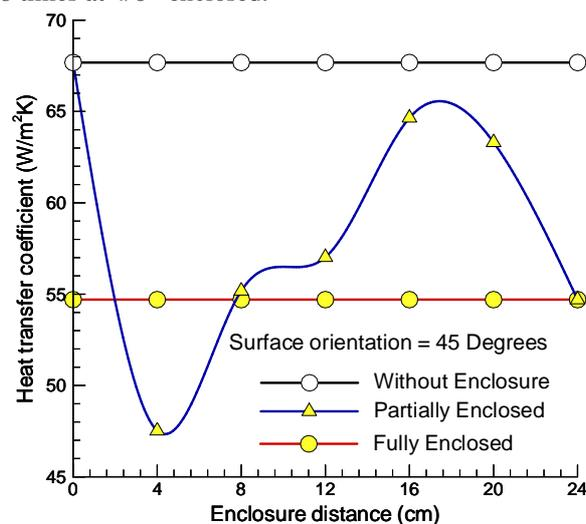
**Figure 9** Variation of heat transfer coefficient with enclosure distance for 45° surface orientation.
