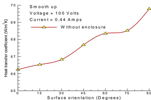
**Figure 3** Variation of heat transfer coefficient with surface orientation for smooth surface facing upward.
