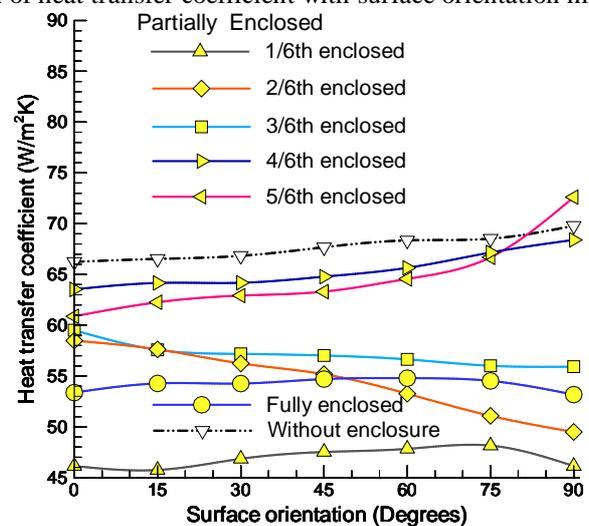
**Figure 6** Variation of heat transfer coefficient with surface orientation for complete enclosure effect
