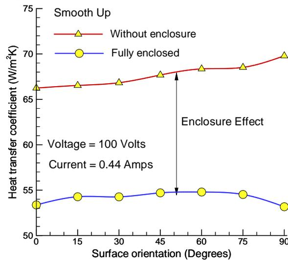
**Figure 5** Variation of heat transfer coefficient with surface orientation highlighting enclosure
