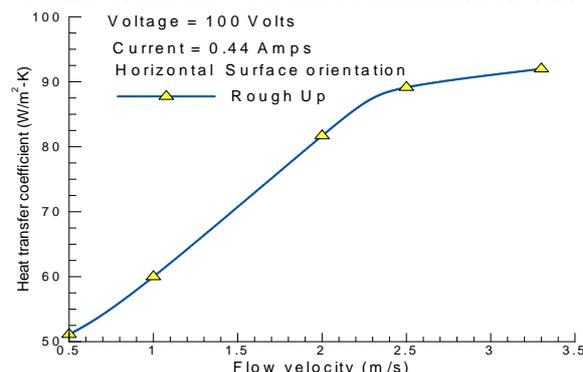
**Figure 4** Variation of heat transfer coefficient with flow velocity and surface for rough surface facing upward.
