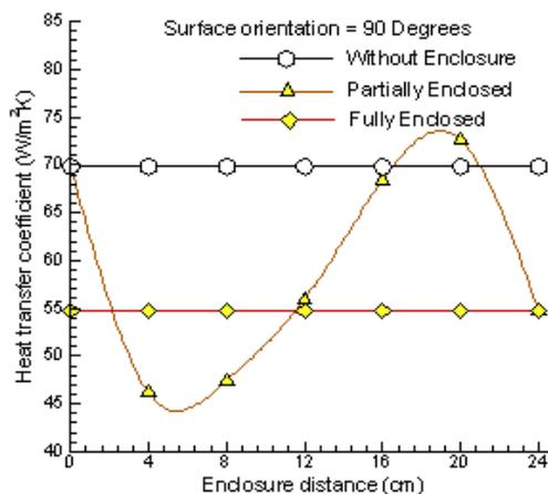
**Figure 7** Variation of heat transfer coefficient with enclosure distance for vertical orientation.
