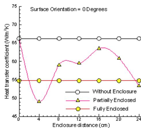
**Figure 8** Variation of heat transfer coefficient with enclosure distance for horizontal orientation.
