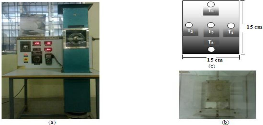
**Figure 1** Pictorial view of the apparatus (a) Front view (b) Top view of square plate (c) schematic of square plate with location of embedded equidistant thermocouples (shown by circles).
