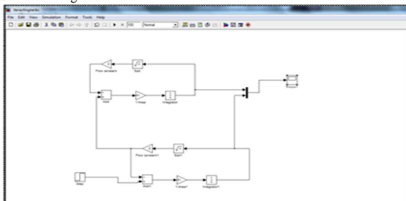
**Figure13** Simulink diagram for Interacting Tank System
