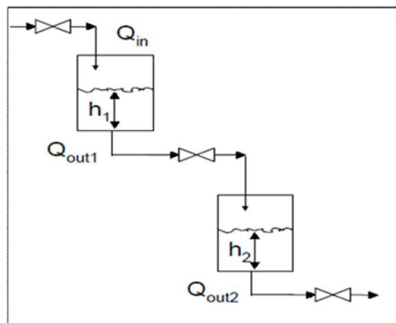
**Figure 6** Non Interacting tank system
