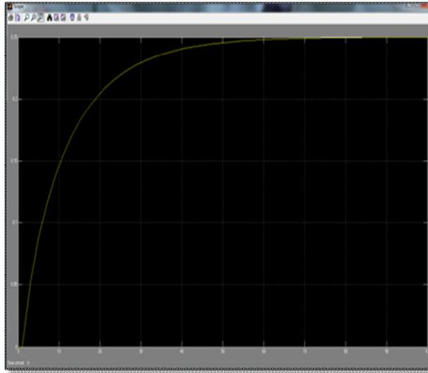
**Figure 4.** Response of Single Tank System
