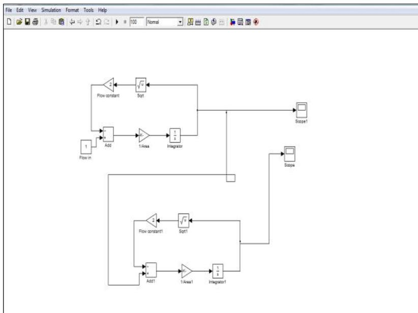
**Figure 7** Simulink diagram for Non-Interacting Tank System
