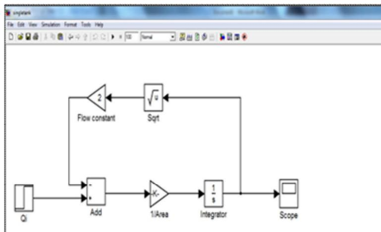
**Figure 3** Simulink Diagram for Single Tank System
