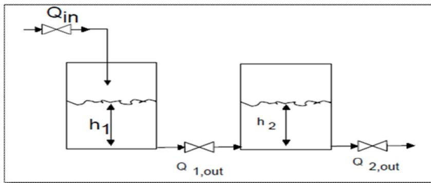
**Figure 12** Interacting Tank System
