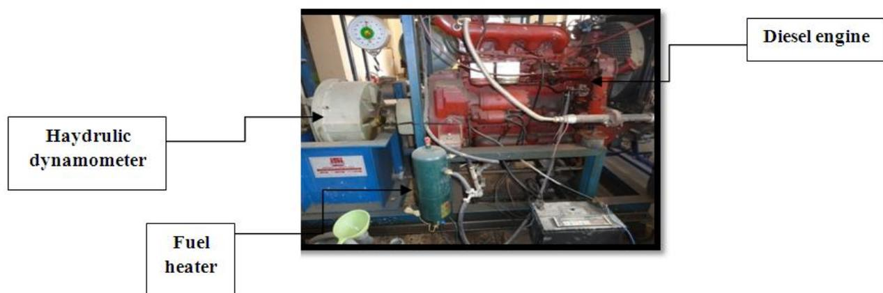
**Figure (1), C.I. engine experimental rig**
