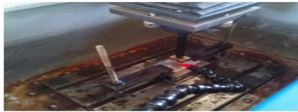
**Fig.2** Electrode setup
