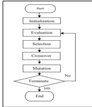
**Fig. 1:** Flow of Standard Genetic Algorithm [17]
