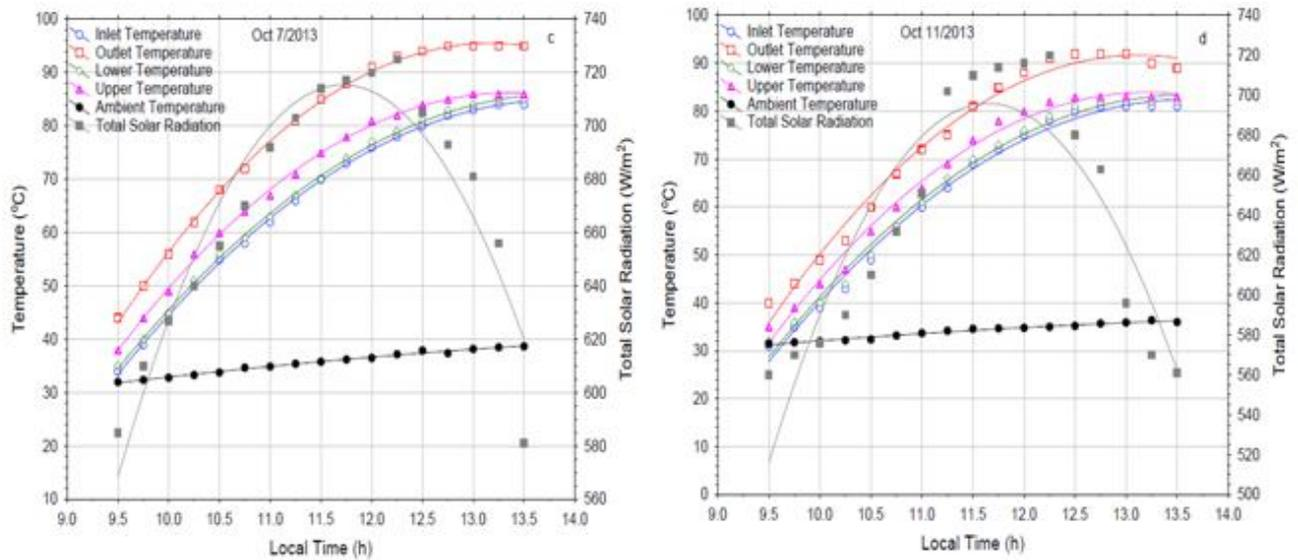
**Figure 5,a,b,c&d:** show variation of total solar radiation and history temperatures of PTSC for different clear October days.
