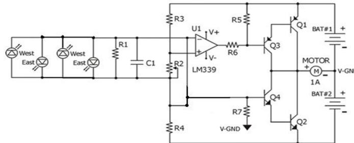
**Figure 4:** circuit diagram of tracking system.
