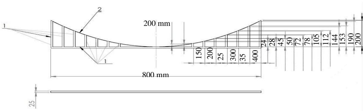
**Figure 3:** Schematic of reflecting base parts (1) steel tubes (2) steel flat bar.
