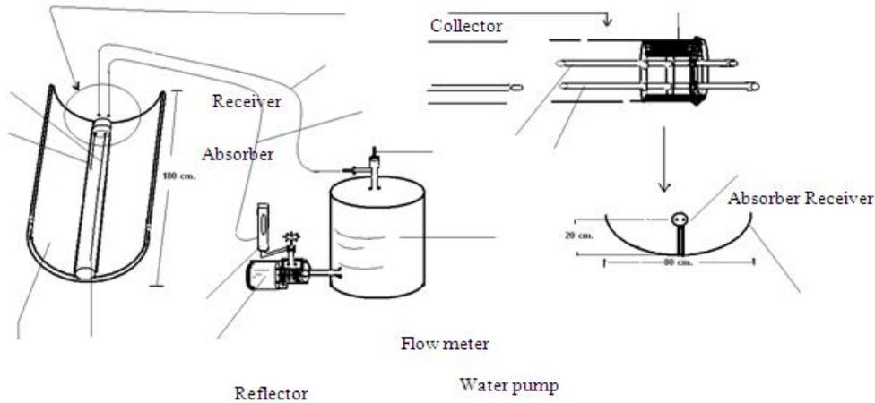
**Figure 1:** Schematic diagram of the PTSC.
