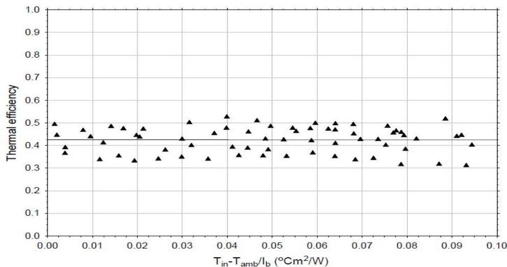
**Figure 7:** Thermal efficiency curve for PTSC.
