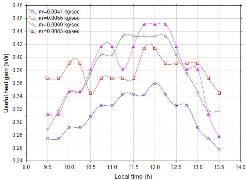
**Figure 6:** Variation of  $Q_u$  with time for different flow rates at October month
