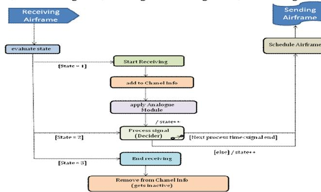
**Figure 5** Synchronized Scheduling in Data Transmission Supported in OMNETPP
