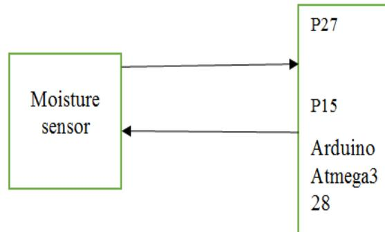
Figure 5 Soil moisture interfacing to MC
