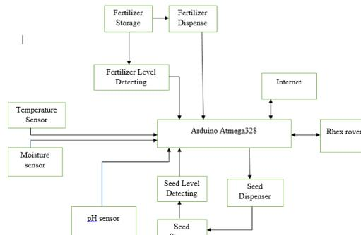
**Figure 1** block diagram of robot
