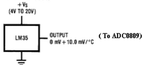
Figure 3 LM35 connected to ADC0809
