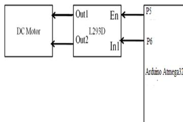
Figure 5 DC motor interfacing to MC
