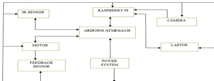
**Figure 2** Block diagram of Rhex rover
