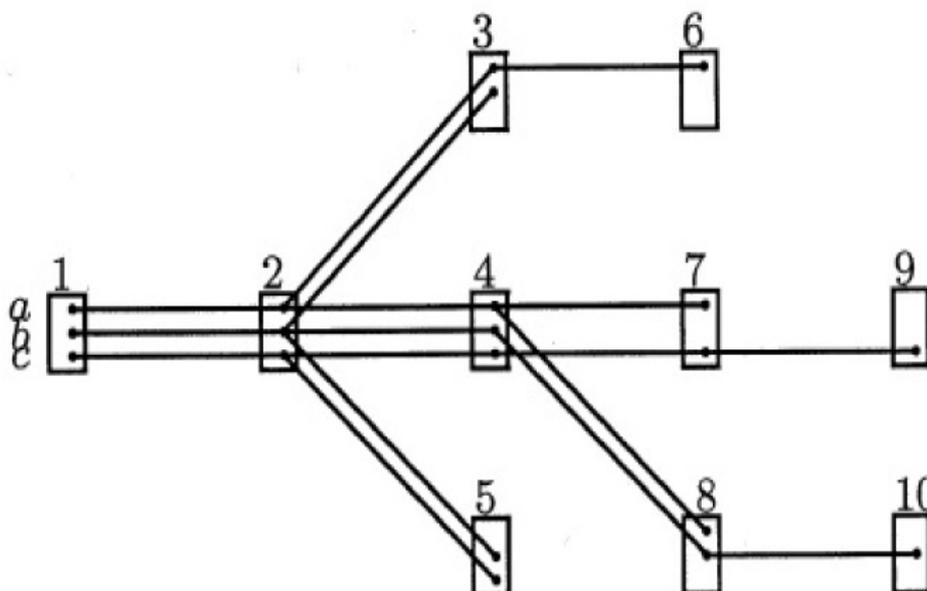
Figure 2: Line diagram of the 10-node unbalanced distribution network
