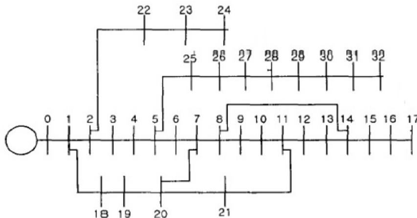
**Figure 1:** Line diagram of the 33-node balanced distribution network
