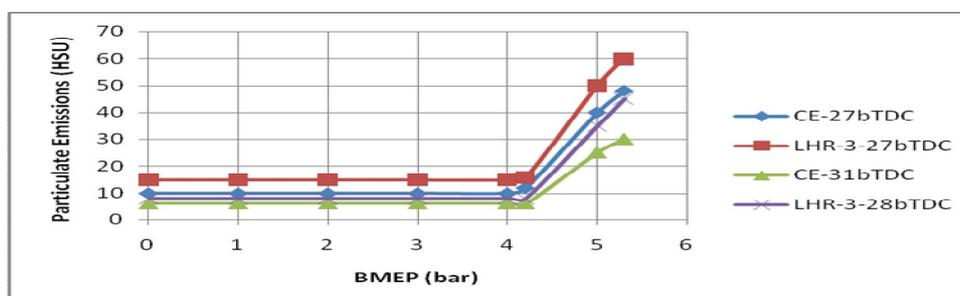
**Figure.5.** Variation of particulate emissions in Hartridge Smoke Unit with brake mean effective pressure (BMEP) with engine with both versions of the combustion chamber at recommended and optimized injection timing.
