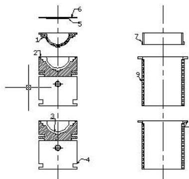
**Figure.1.** Schematic diagram of assembly the insulated piston, insulated liner and ceramic coated cylinder head of the engine with LHR–3 combustion chamber .
