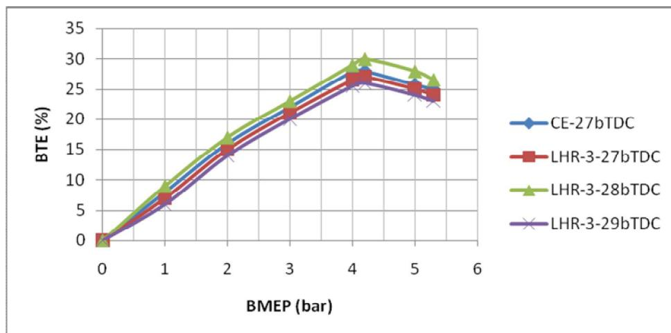
**Figure.4.** Variation of brake thermal efficiency (BTE) with engine with LHR-3 combustion chamber with neat diesel, at various injection timings at an injector opening pressure of 190 bar.
