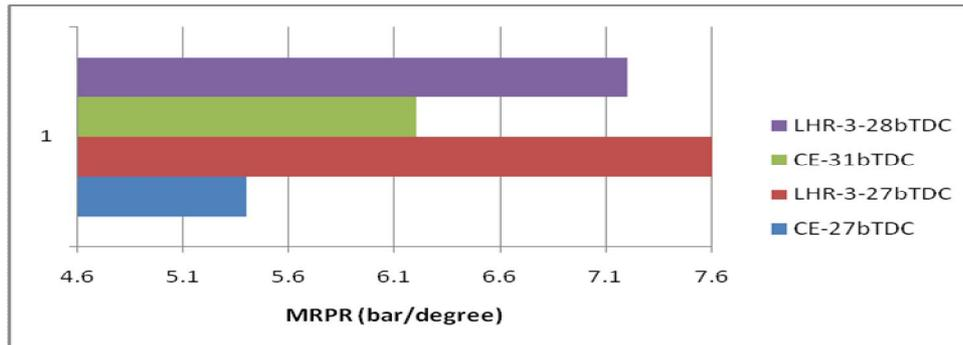
**Figure.10** Bar charts showing the variation of maximum rate of pressure rise (MRPR) at full load with injection timing with both versions of the combustion chamber
