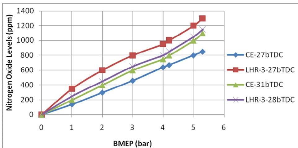
**Figure.7.** Variation of nitrogen oxide levels with brake mean effective pressure (BMEP) with engine with both versions of the combustion chamber at recommended and optimized injection timing.
