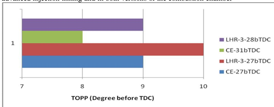
**Figure.11** Bar charts showing the variation of time of occurrence of peak pressure (TOPP) at full load with injection timing with both versions of the combustion chamber
