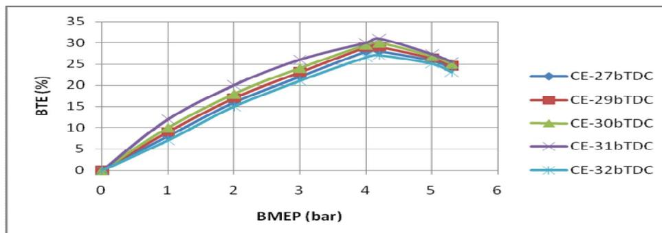
**Figure.3** variation of brake thermal efficiency (BTE) with brake mean effective pressure (BMEP) in the conventional engine with neat diesel, at various injection timings at an injector opening pressure of 190 bar.
