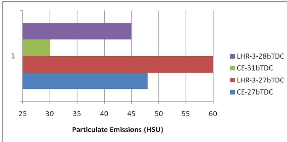
**Figure.6.** Bar charts showing the variation of particulate emissions at full load with injection timing with both versions of the combustion chamber
