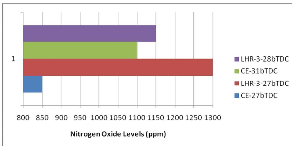
**Figure.8.** Bar charts showing the variation of nitrogen oxide levels at full load with injection timing with both versions of the combustion chamber
