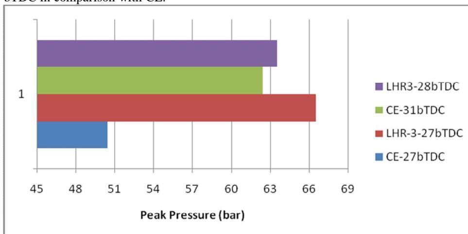
**Figure.9** Bar charts showing the variation of peak pressure at full load with injection timing with both versions of the combustion chamber
