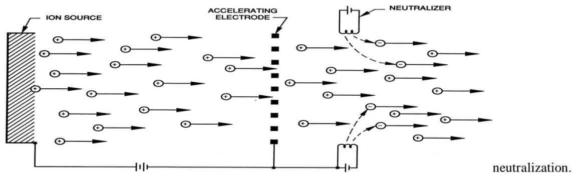
**Figure : 4 - Ion thruster schematic**
