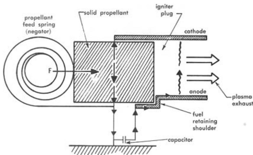
**Figure : 8-** Pulsed Plasma Thruster
