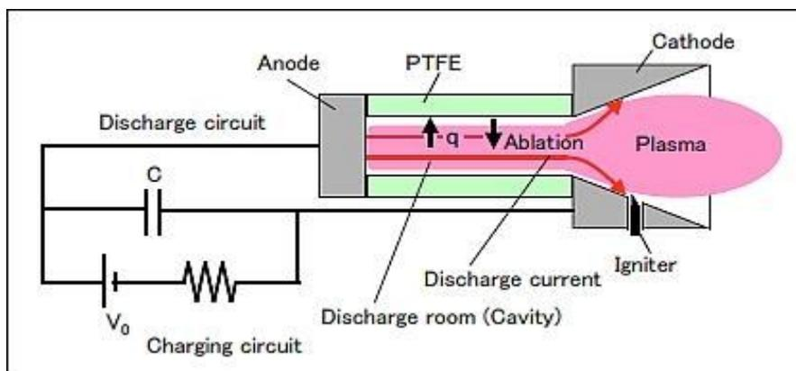
**Figure :9-** Schematic view of the PPT
