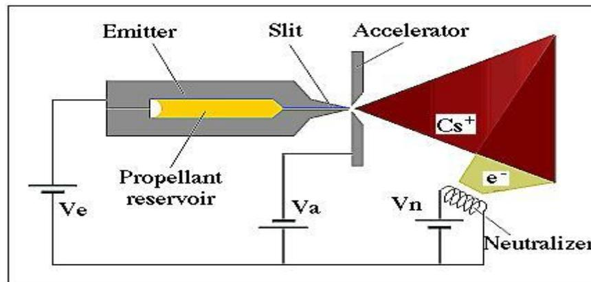
**Figure : 5 - Colloid thruster schematic**
