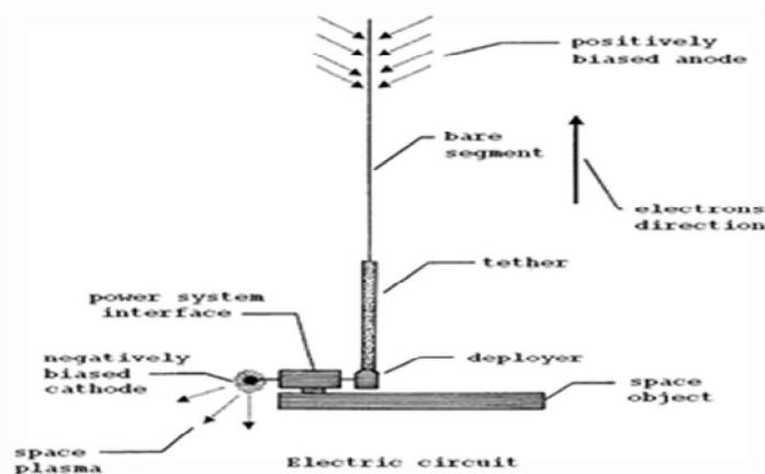
**Figure : 10-** Electrodynamic Tether
