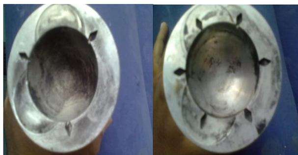
**Fig. 2** Different types of configurations of piston crowns
