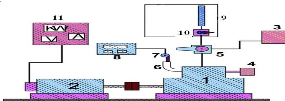
Fig 1 Experimental Setup of the Test Engine
