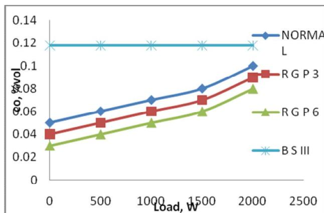
**Fig. 7 Load Vs Carbon monoxide**
