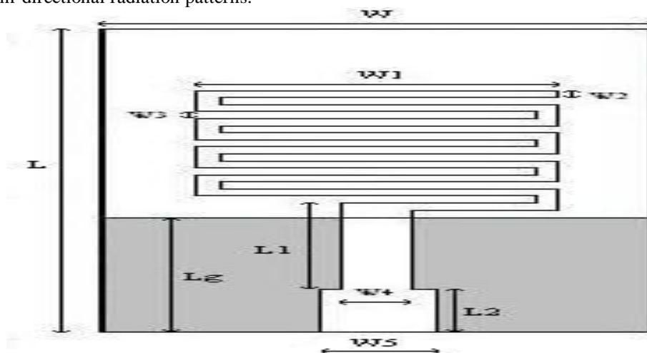
**Fig. 1.** Geometry of the single Meander Line ESA.
