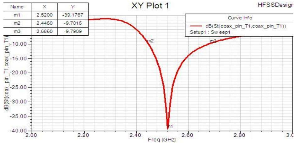
**Fig.3** Simulated return loss for proposed MLA antenna
