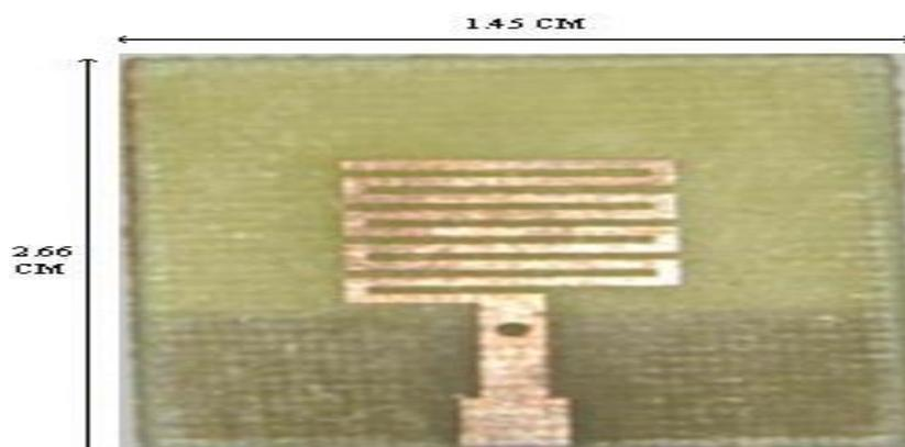
**Fig.2** Photo of the fabricated antenna
