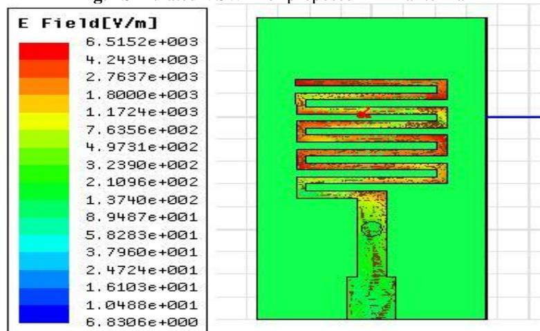
**Fig.5** Surface current distribution on MLA at 2.52 GHz
