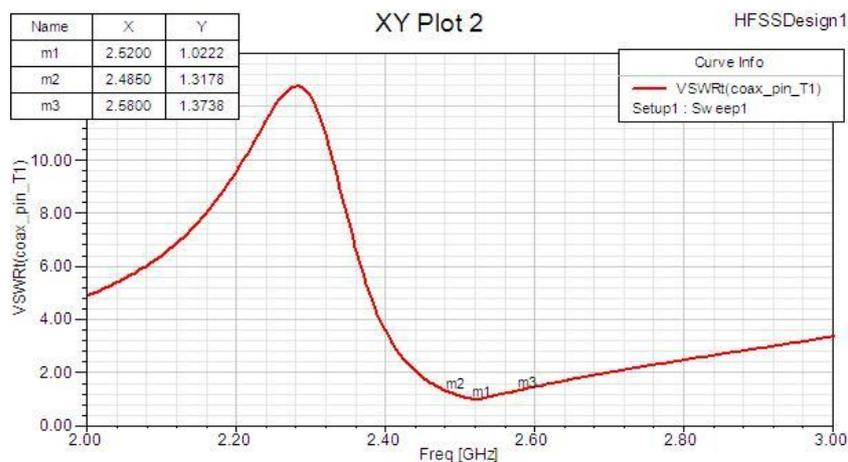
**Fig.4** Simulated VSWR for proposed MLA antenna
