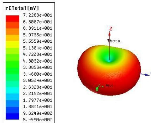
**Fig.6 (a)** Radiation Pattern of Proposed antenna 3D Polar Plot
