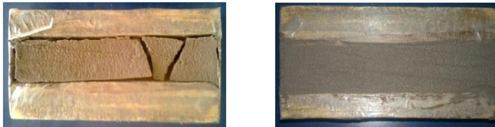
**Figure 11** Shrinkage of 60% black cotton soil + 40% Brick dust
