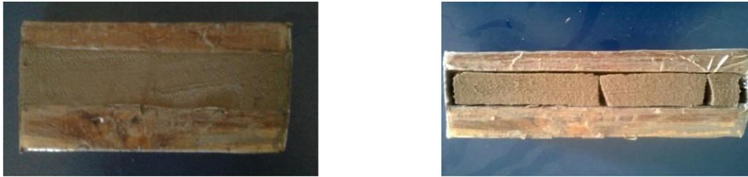
**Figure 10** Shrinkage of 60% black cotton soil + 40% marble powder
