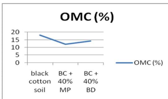
**Figure 8** graph for optimum moisture content
