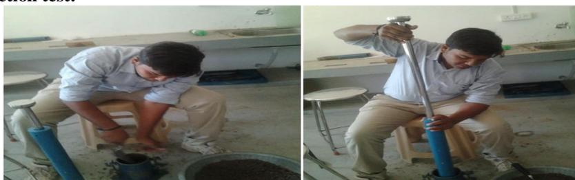
**Figure 6** Determination of maximum dry density and optimum moisture content
