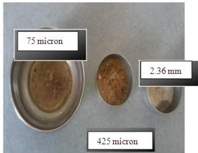
**Figure 3** Samples from wet sieve analysis
