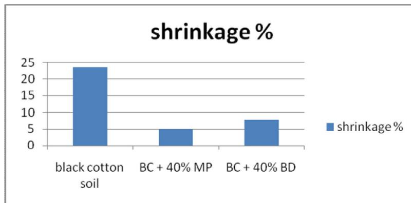
**Figure 12** graph for linear shrinkage
