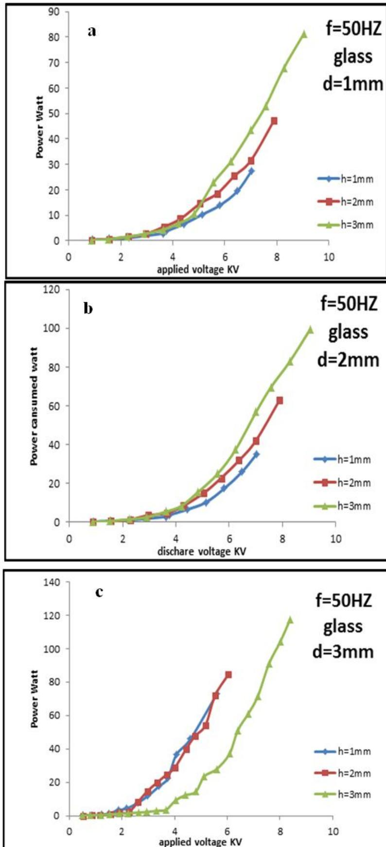
Fig.4(a,b,c) shows the power consumed in DBD system as a function of discharge voltage for three different gap space,  $h$  (1,2,3) mm and three values of glass thickness  $d$  (1,2,3) mm.
