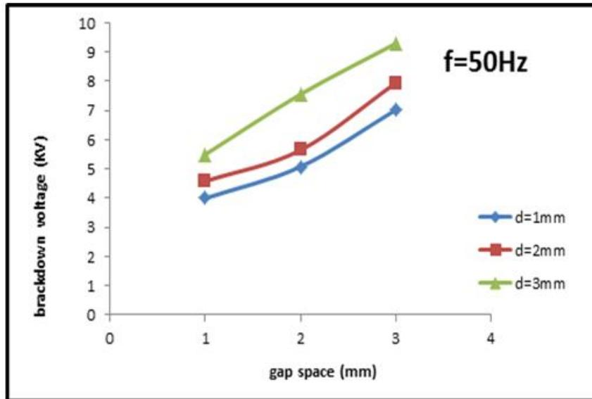
**Figure. 6.** shows breakdown voltage of DBD system as a function of gap space for different glass thickness, d (1, 2,3) mm. and frequency, f (50)Hz
