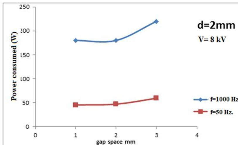
**Fig .10.** Power consumed in DBD system as a function of gap space for two different frequency (50, 1000) Hz in glass thickness, d (2) mm.
