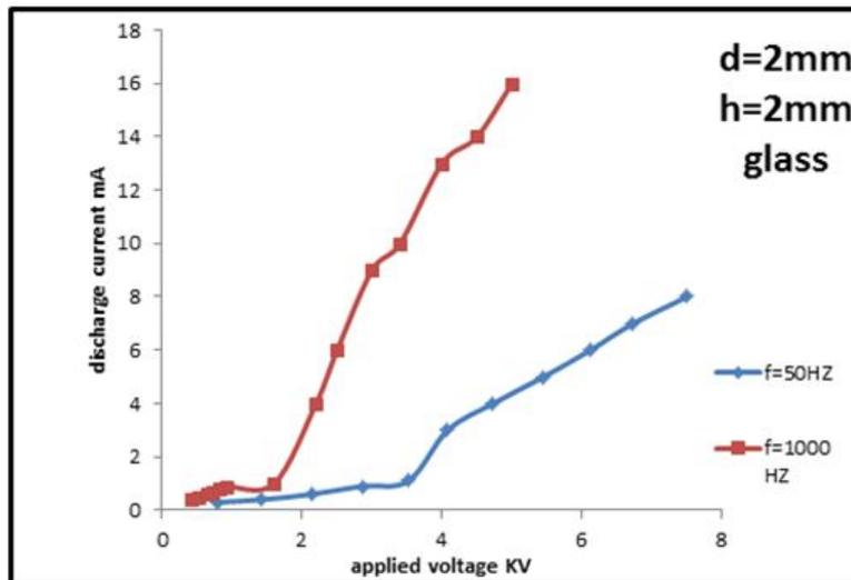
**Fig.7.** shows discharge current as a function of voltages for two frequencies in glass thickness, d (2) mm. and gap space, h (2) mm.
