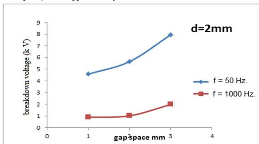
**Figure. 9.** shows breakdown voltage as a function of gap space for two frequencies (50,1000) Hz. in glass thickness, d (2)mm.
