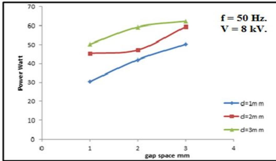
**Fig .5.** Power consumed in DBD system as a function of gap space for three different glass thinness (1,2,3) mm.
