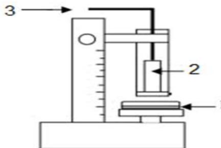
**Figure 1:** Schematic setup for of parallel plate DBD (1)glass layer (2) copper electrode (3) High voltage.
