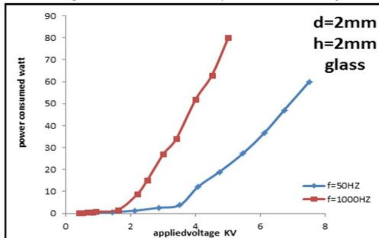
**Fig .8.** Power consumed in DBD system as a function of discharge voltage for two values of frequency (50, 1000) Hz. in glass thickness, d (2) mm. and gap space, h (2) mm
