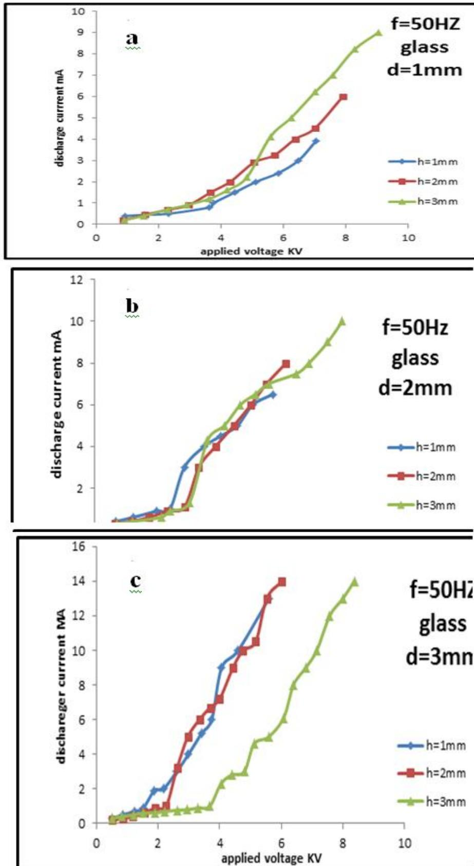
Fig.3.(a,b,c) shows the discharge current as a function of applied voltage with glass thickness d(1,2,3) mm, for three gap space, h(1,2,3) mm.
