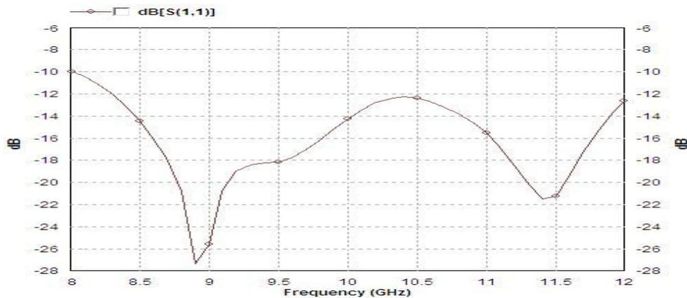
**Figure 9** Return loss for the reflector design
