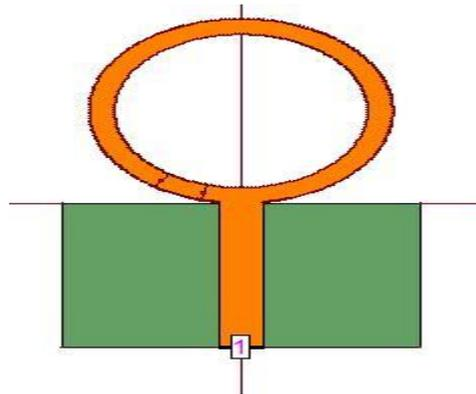
**Figure 1** Geometry of monopole Antenna.
