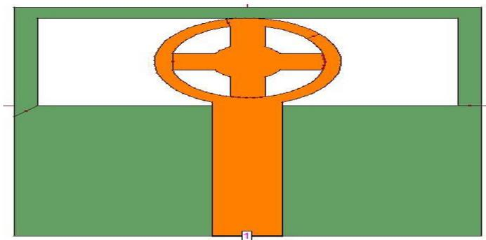
**Figure 6** Compact monopole antennas with reflector
