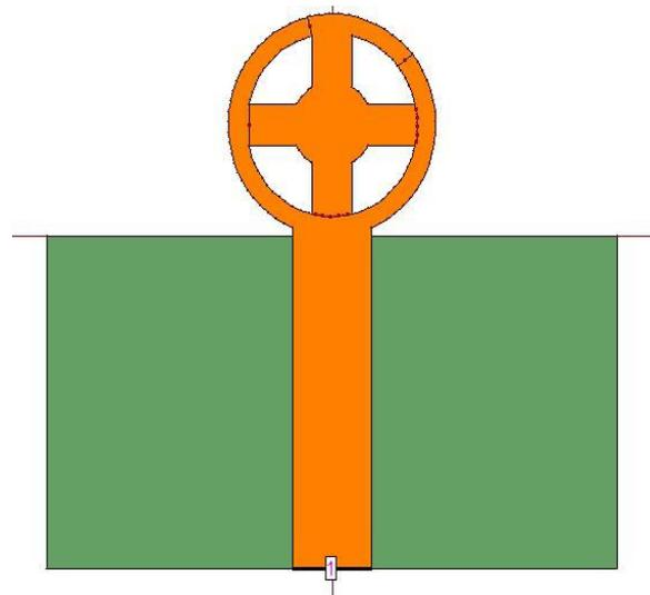
**Figure 3** Geometry of compact circular cross spoke monopole Antenna.
