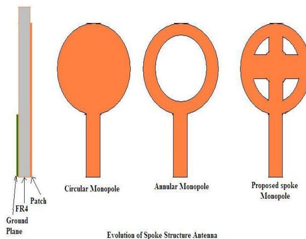
**Figure 2** Proposed shape X band antenna
