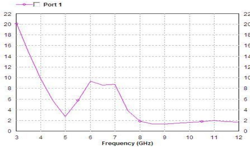
**Figure 8** VSWR graph of compact monopole antenna with reflector
