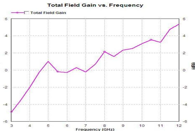
**Figure 7** Gain graph of Compact Monopole Antenna with Reflector
