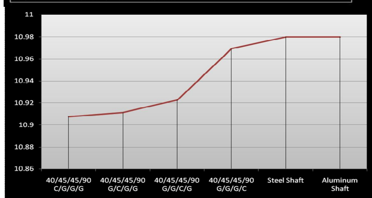
Fig. Comparison of Composite Shaft with Metal Shafts for Torsional Shear Stress
