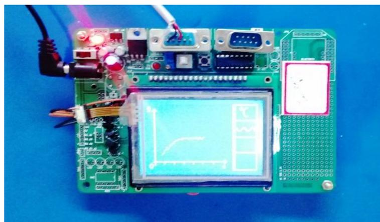
**Fig.6:** Master node displaying voltage levels in graphical form
