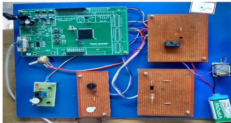
**Fig.4:** Data acquisition node with sensors
