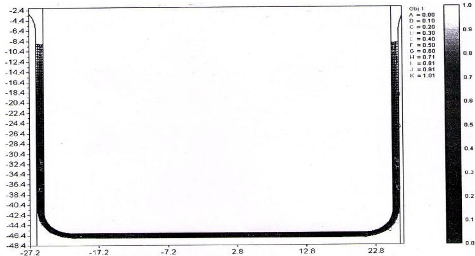
**Fig.5** Effective strains contours in the successfully formed cup
