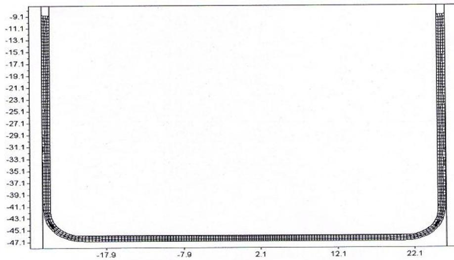
Fig.3 Finite element analysis mesh of successfully drawn cup
