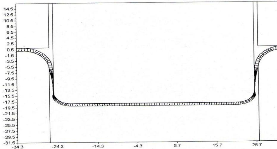
Fig.2 Fracture at corners during the cup formation with further advancement of the punch into the sheet material
