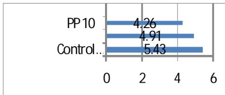
**Graph 1:** Comparison of Aggregate Impact Value Test Results
