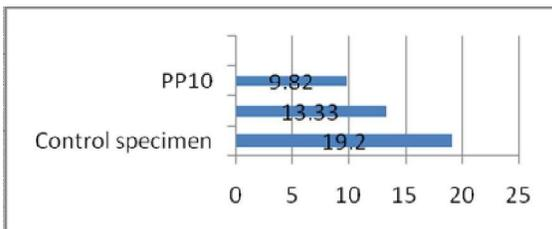
**Graph 2:** Comparison of Aggregate Crushing Value Test Results
