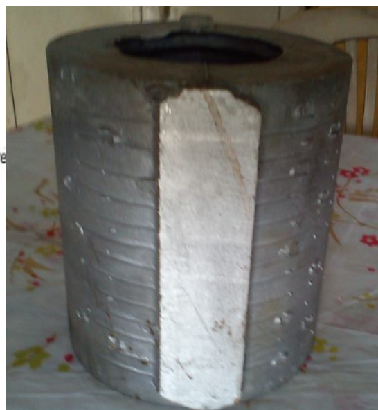
Fig. 1.2 Defected Shell Core Drum
