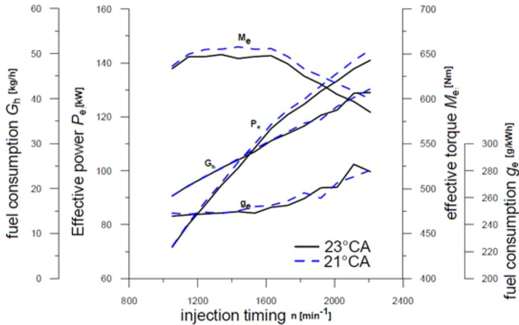
Figure 3: Effective power  $P_e$ , effective torque  $M_e$ , fuel consumption  $G_h$  and specific fuel consumption  $g_e$  for use of bio diesel fuel with injection timing of 21°CA and 23°CA before TDC
