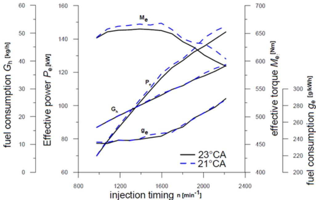
**Figure 4:** Effective power  $P_e$ , effective torque  $M_e$ , fuel consumption  $G_h$  and specific fuel consumption  $g_e$  for use of diesel fuel with injection timing of 21°C A and 23°C A before TDC
