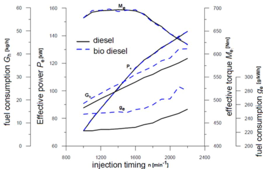
**Figure 1:** Effective power  $P_e$ , effective torque  $M_e$ , fuel consumption  $G_h$  and specific fuel consumption  $g_e$  for use of diesel and bio diesel fuels with injection timing of 23°CA before TDC
