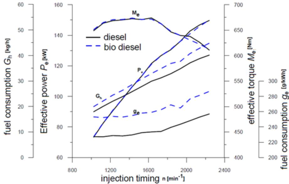
Figure 2: Effective power  $P_e$ , effective torque  $M_e$ , fuel consumption  $G_h$  and specific fuel consumption  $g_e$  for use of diesel and bio diesel fuels with injection timing of 21°CA before TDC
