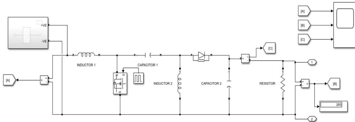
Fig. 3.3 SIMULINK model of PV based SEPIC Converter
