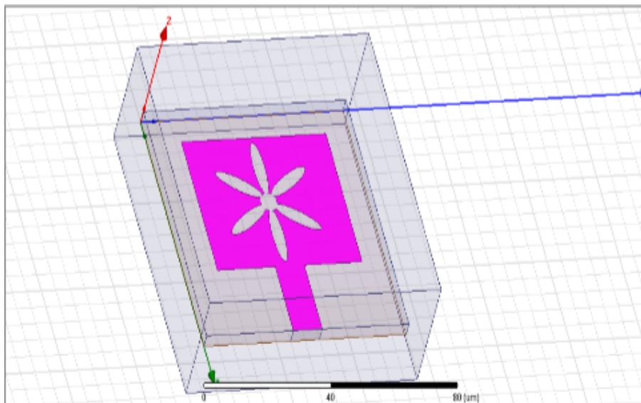
Fig. 2: The proposed micro strip antenna designed in the HFSS software
