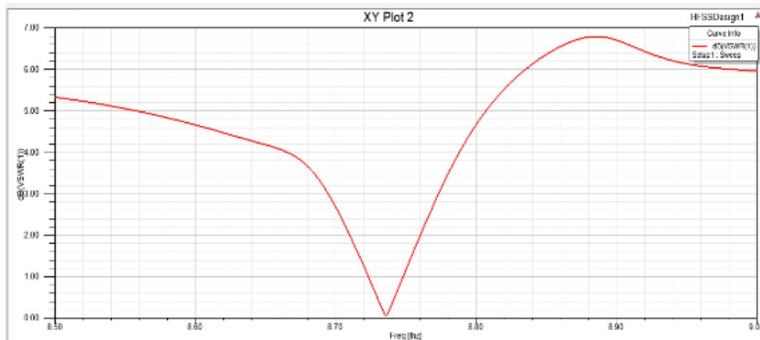
Fig. 4: VSWR vs frequency plot of the proposed micro strip antenna
