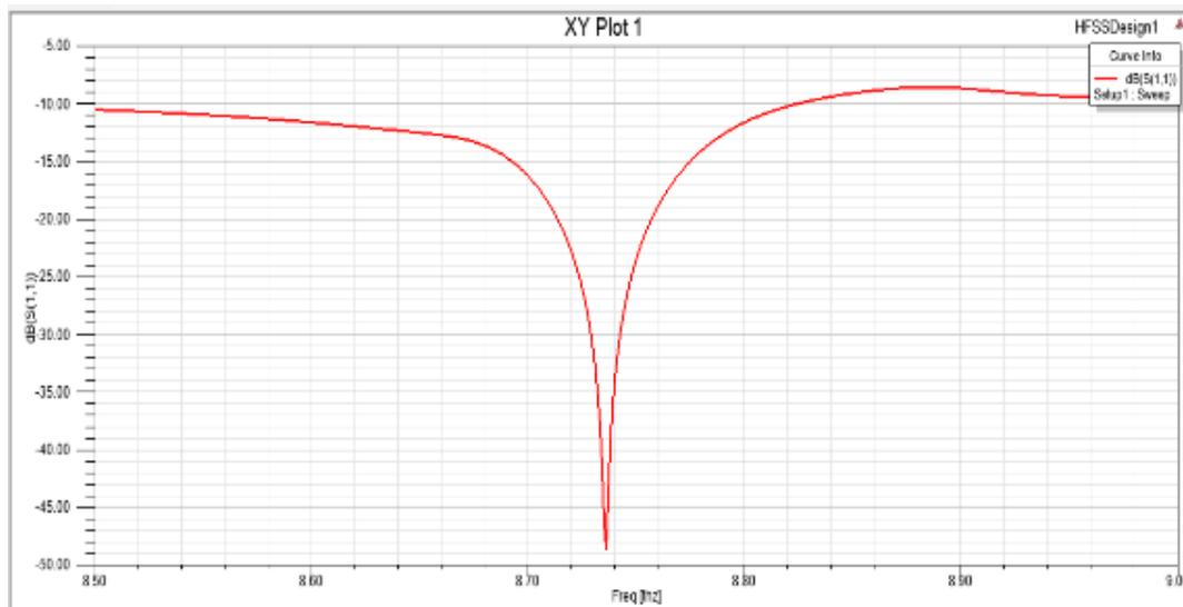
Fig. 3: S11 vs frequency plot of the proposed micro strip antenna
