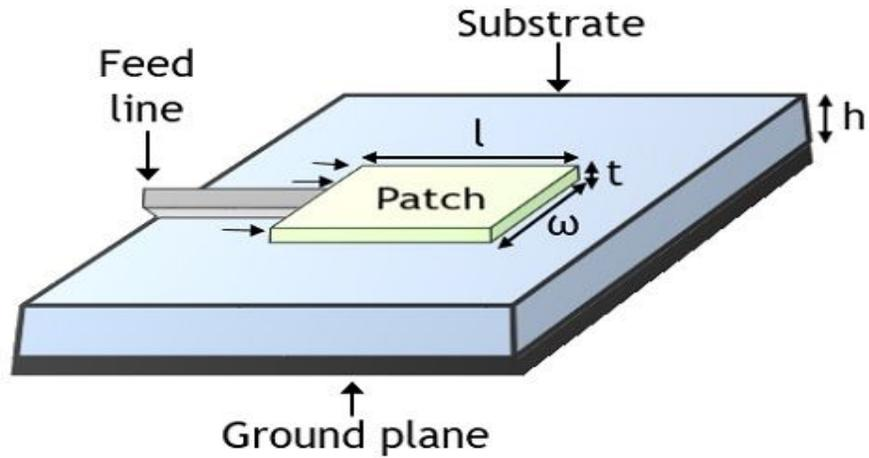
Fig.1: A general overview of Micro strip patch antenna
