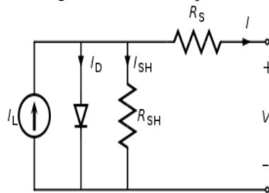
**Fig.1:**Equivalent circuit of Ideal PV cell
