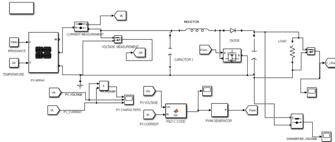
**Figure.6:** Simulink Model of P&O MPPT with dc-dc converter
