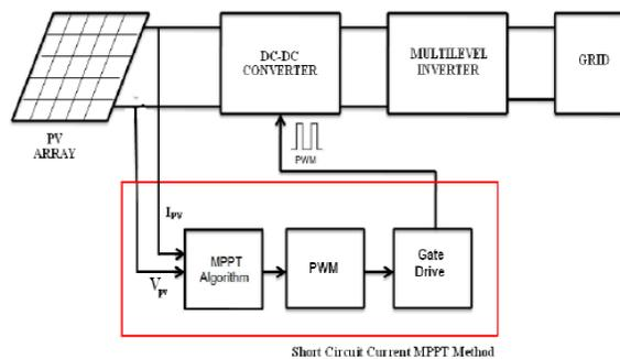
**Fig.3:** System configuration of PV System
