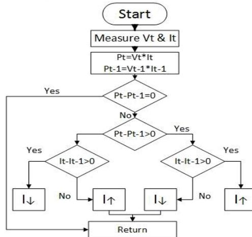
**Fig.4:** Flowchart of P&O Algorithm
