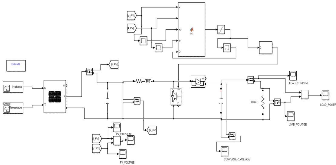
**Figure.8:** Simulink Model of InC MPPT with dc-dc Converter
