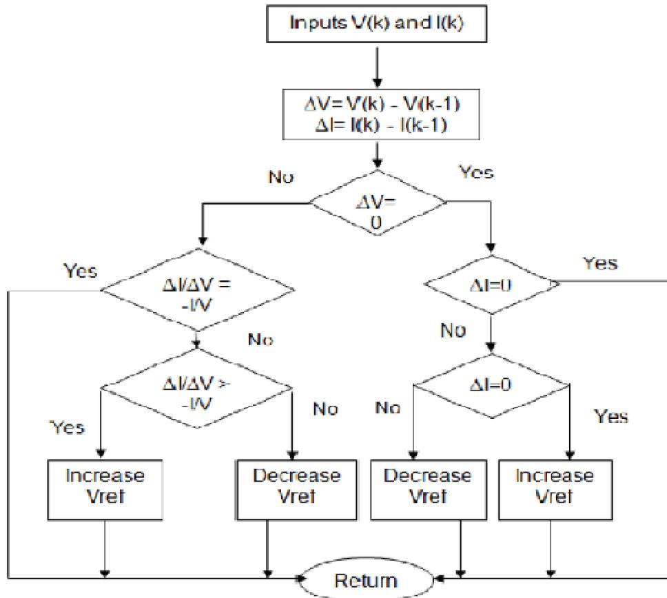
Fig.5:Flowchart of Incremental conductance method
