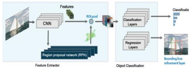
**Figure 6** Faster R-CNN Detector [ 16].
