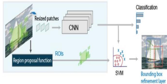
**Figure 4** R-CNN Detector [16].
