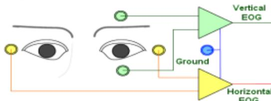
Figure 1: Correct positions of five electrodes [10]
