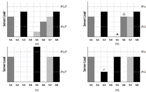
**Figure4.** Server load scenario: a) S5 is under PoT b) S5 switched off and VMs migrated to S6 c) S5 above WoT d) S3 is switched on.
