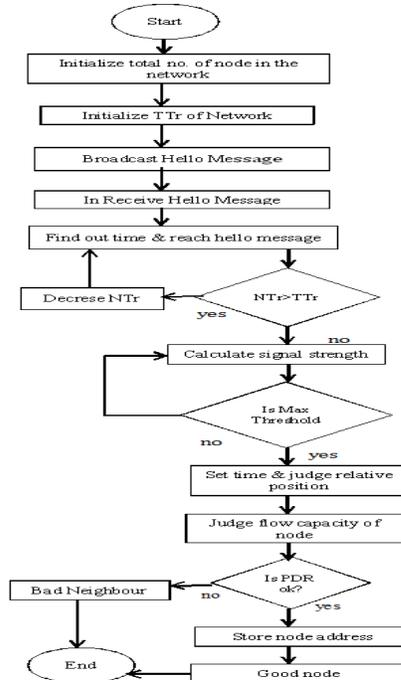
Figure 1.Process Flow of GNDA
