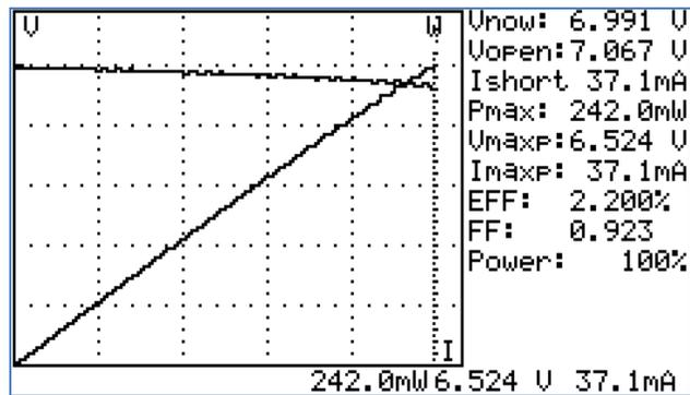
**Figure 2:** Current-Voltage curve solar cell using LSC Chlorophyll ( $8.42 \times 10^{-3}$  mol/L) with 1mm thickness
