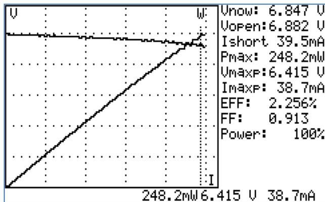
**Figure 3:** Current-Voltage curve solar cell using LSC Chlorophyll ( $8.42 \times 10^{-3}$  mol/L) with 0.75 mm thickness
