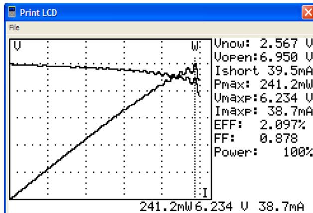
**Figure 1:** Current-Voltage curve solar cell using LSC Chlorophyll (8.4298x10<sup>-3</sup> mol/L) with 2mm thickness
