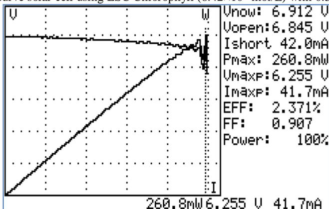
**Figure 5:** Current-Voltage curve solar cell using LSC Chlorophyll ( $8.42 \times 10^{-3}$  mol/L) with 0.25 mm thickness.
