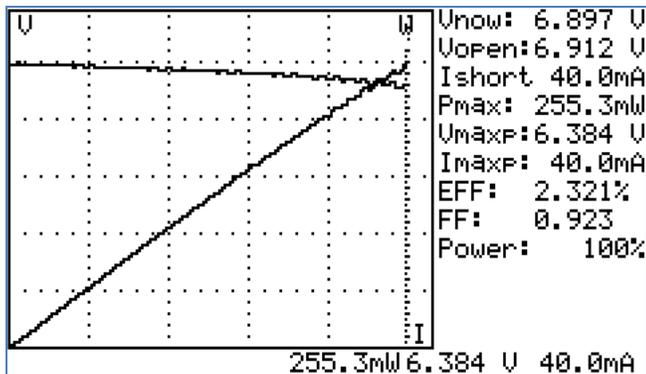
**Figure 4:** Current-Voltage curve solar cell using LSC Chlorophyll ( $8.42 \times 10^{-3}$  mol/L) with 0.5 mm thickness
