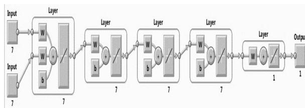
**Fig. 2:** Custom designed Back Propagation Neural Network (BPNN) model for STLP for SPDCL of A.P.
