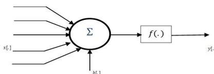
**Fig. 1:** A single artificial neuron model
