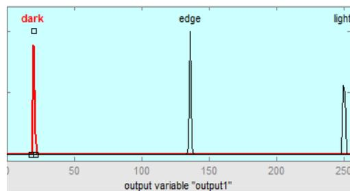
**Figure 2** Membership functions of the fuzzy set associated to the input
