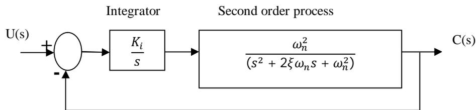
Figure 1 Block diagram of third order process simulator
