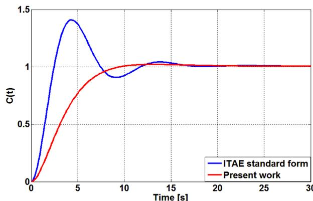
Figure 5 Comparison of Step response of the PD-PI controlled third order process tuned by ITAE standard form and ISTSE
