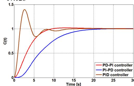
Figure 6 Step response of the third order process controlled by PD-PI, PI-PD and PID controllers
