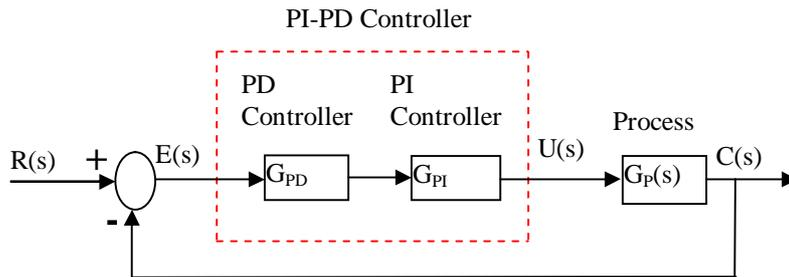
Figure 3 PD-PI controller-based control system
