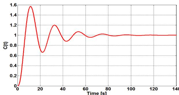
Figure 2 Step response of the uncontrolled third order process
