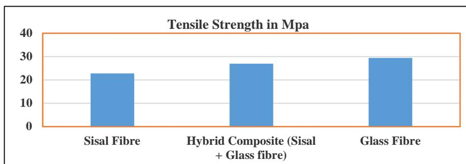
Fig 3. Tensile strength of Sisal/Glass fibre composites and hybrid composite.
