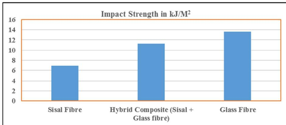
Fig 6. Impact strength of Sisal/Glass fibre composites and hybrid Composites.
