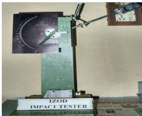
**Fig 2.** Izod Impact testing machine
