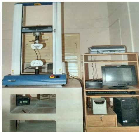
**Fig 1.** Universal testing machine
