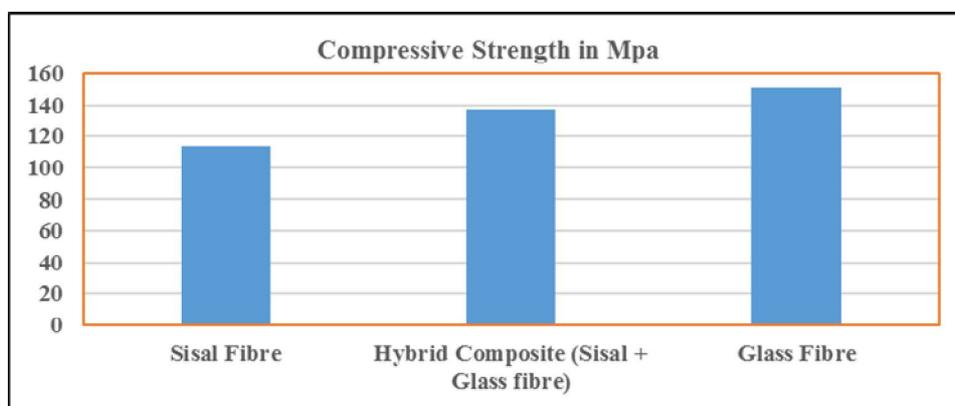
Fig 4. Compressive strength of Sisal/Glass fibre composites and hybrid composite.
