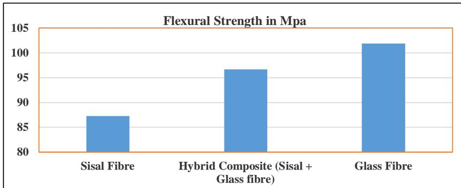
Fig 5. Flexural strength of Sisal/Glass fibre composites and Hybrid composite.
