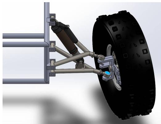
**Figure 8:** Assembly of Suspension system with roll cage
