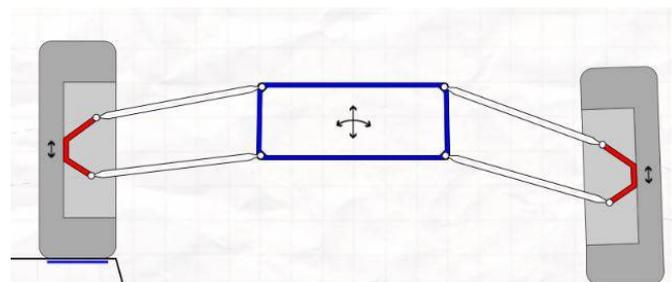
**Figure 6:** Simulation of a wheel during a bump
