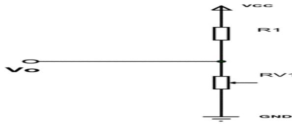
Fig.3 Voltage divider
