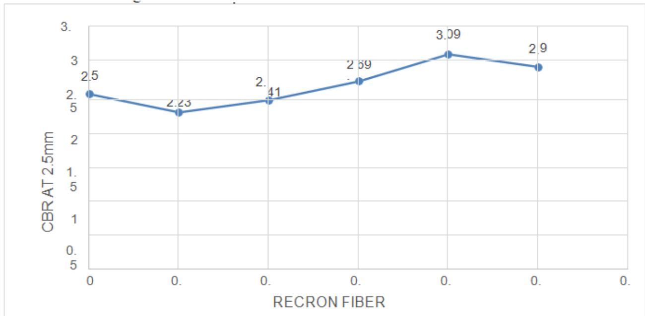
**Fig.5** Variation of CBR 2.5 mm with fiber content
