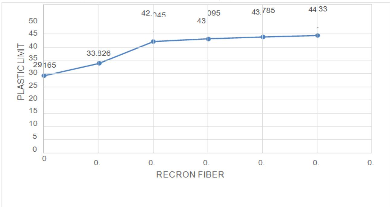
Fig.2 Variation of plastic limit with fiber content
