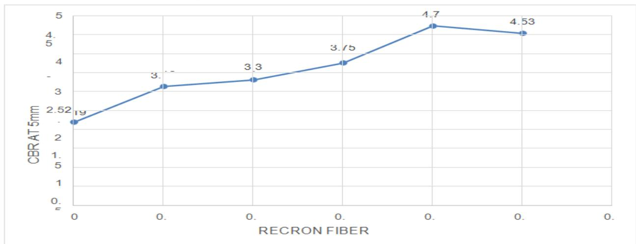
**Fig.6** Variation of CBR 5mm with fiber content
