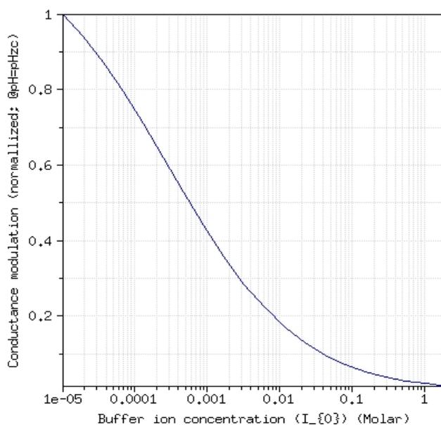
Fig 6 Conductance modulation vs. buffer ion concentration
