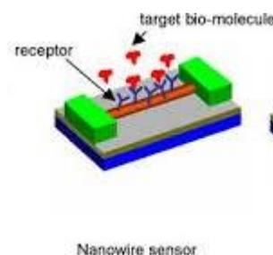
Fig.1. Structure of Cylindrical Nanowire sensor[5]
