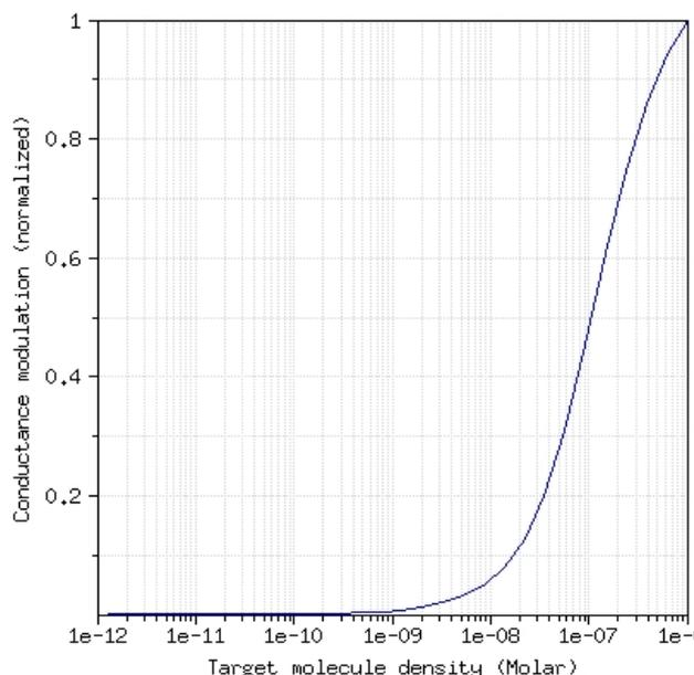
Fig 5 Conductance modulation vs. target molecule density
