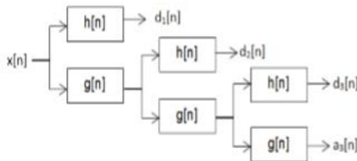
**Figure 3** Three Level Wavelet Decomposition tree
