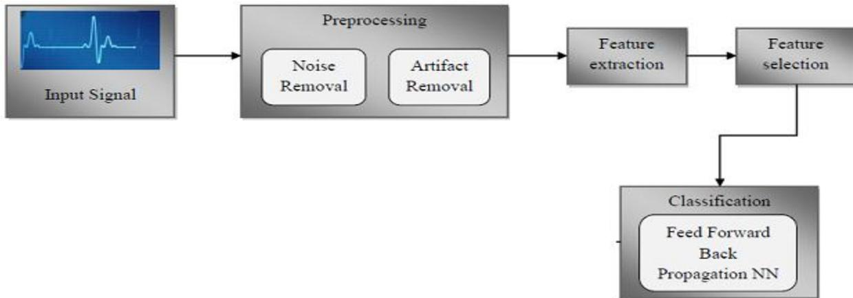
**Figure 2** Block Diagram for Classification Methodology.
